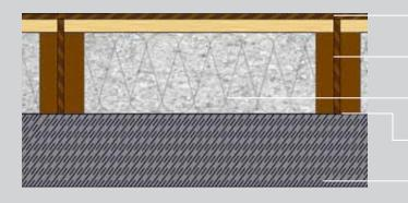
OSB 3 board WoodyFIX basic module ISOCELL cellulose insulation Vapour barrier <sup>2)</sup> Concrete floor
